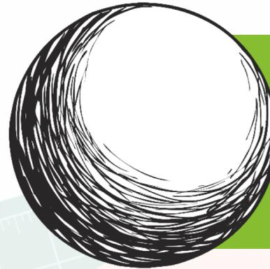
**Contour-hatching** follows the contour, or curve or outline, of the object. In this case, the hatching is rounded to match the shape of the circle.
